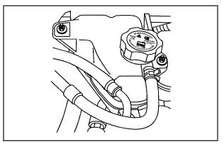
The engine coolant surge tank is located in the rear of the engine compartment. See *Engine Compartment Overview on page 352* for more information on location.
